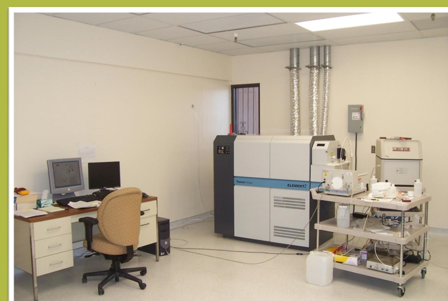
Fig. 3. The Nine Circles Analytical Cosmochemistry laboratory equipped with the Thermo Finnigan Element2 ICP-MS (on the left) coupled with the CETAC LXS-213 Nd:YAG laser ablation unit (on the right).
