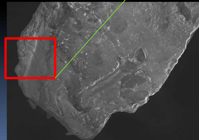
Detail, Ossendrecht quartz grain, SEM, not acid etched
