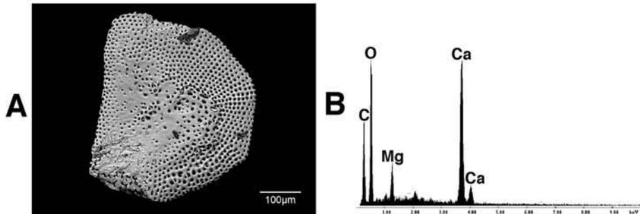
Fig. 13. Marine carbonate fossil. A: SEM image of marine fossil. B: X-ray analysis of composition of fossil. Note that there is a strong Mg peak, consistent with either aragonite or high Mg calcite. The carbonate contains about 26 mol% Mg
