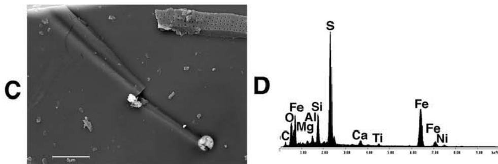
Fig. 20. Pyrite spherule indenting basaltic glass. A: SEM image of entire grain. Pyrite spherule is colored red. B: X-ray analysis of the composition of the glass. C: Close up of iron sulfide spherule indenting glass. The pyrite is following a single track. The offset of the track is an optical illusion. D: X-ray analysis of the composition of the spherule
