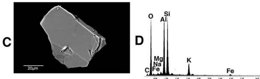
Fig. 19. Possible mineral grains. A: Optically clear pink grain with conchoidal fracture. B: X-ray analysis of the composition of the grain in A. C: Optically clear grain with section peeled back like sardine can. D: X-ray analysis of the composition of the grain in C
