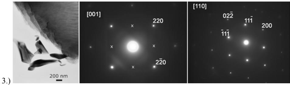
**Figure 3.** Several diamond microflakes alongside amorphous carbon support together with some SAED patterns with extinctions indicated by crosses in  $[001]$  zone.
