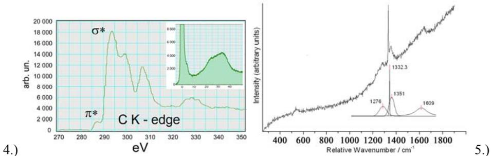
**Figure 4.** C K-edge ELNES revealing characteristic diamond  $\sigma^*$  shape plus plasmon peak at 33 eV in inset.
