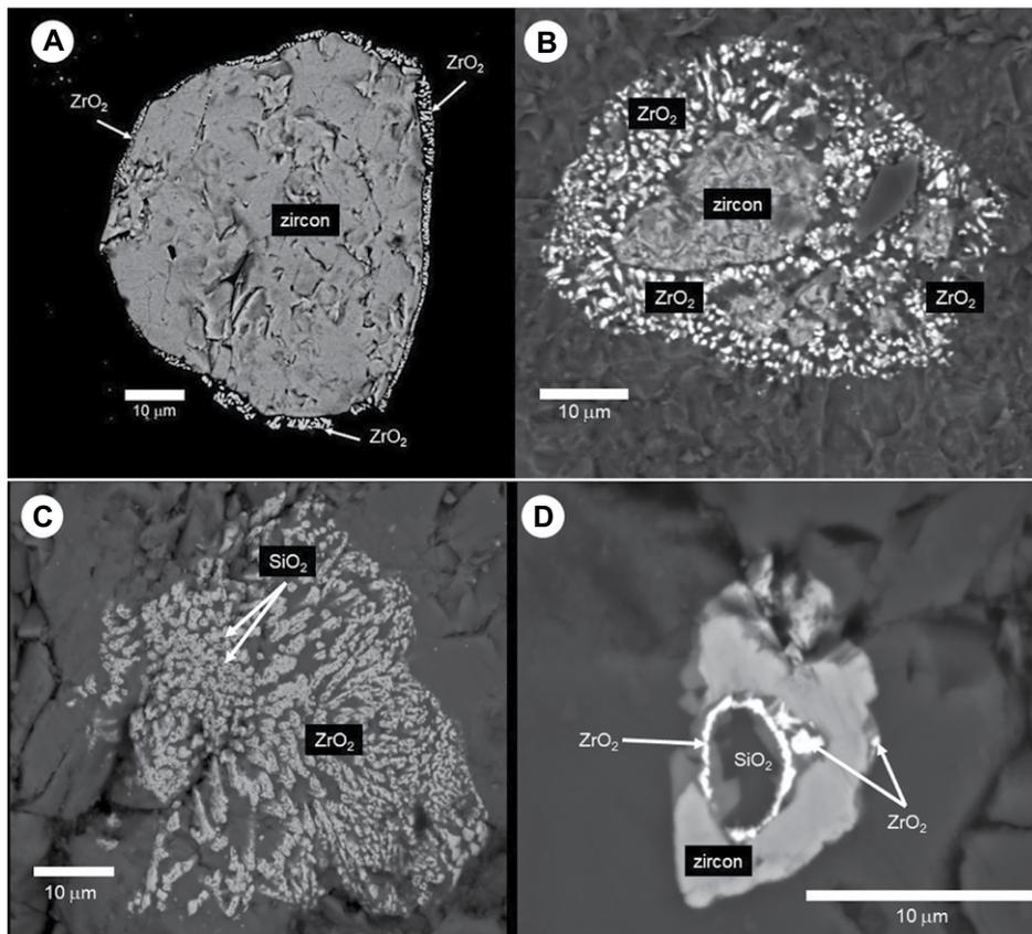
**Figure 3.** Backscattered-electron photomicrographs of zircon inclusions in Pica (Chile) impact glass. Zircon grains exhibit varying degrees of partial (A, B, D) to complete (C) decomposition from  $\text{ZrSiO}_4$  to a  $\text{ZrO}_2$  phase (possibly baddeleyite) and silica. Such thermal decomposition requires temperatures  $>1670^\circ\text{C}$  with rapid quenching.
