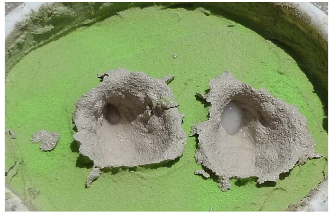
Fig. 5. Impacts by ice projectiles create conical cavities on a viscous surface.
