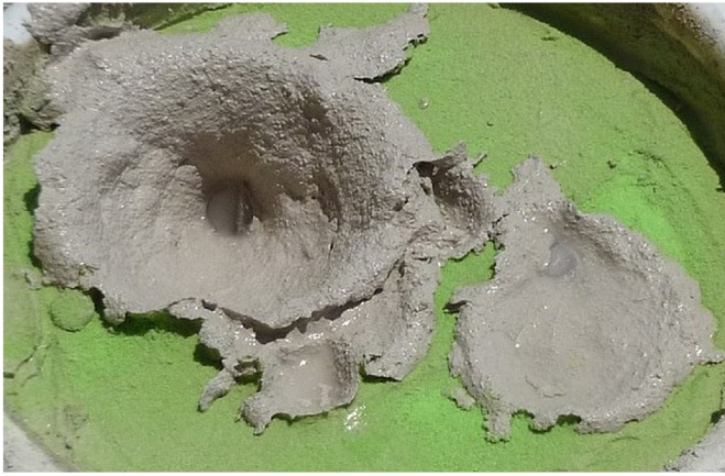
Fig. 7. New impacts make conical cavities without disturbing adjacent bays.
