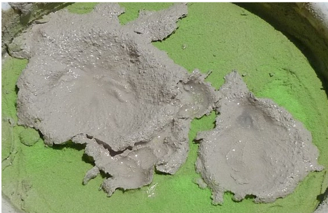
Fig. 8. Viscous relaxation of adjacent conical cavities creates overlapping bays.
