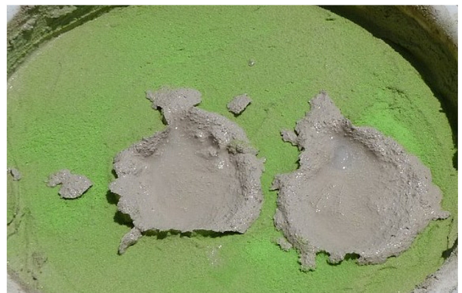
Fig. 6. Viscous relaxation converts conical cavities into shallow bays with raised rims.
